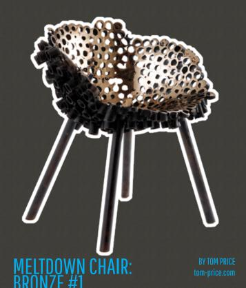
The original form for the chair, made from polypropylene tubes, is encased in a thick ceramic shell and then melted out to create a cavity into which the molten bronze is poured. Once cooled the ceramic shell is broken away to reveal the bronze form within. The back and underside is left 'raw' and patinated black. The seat is polished to a bright mirror finish. Photo credit: James Champion.
